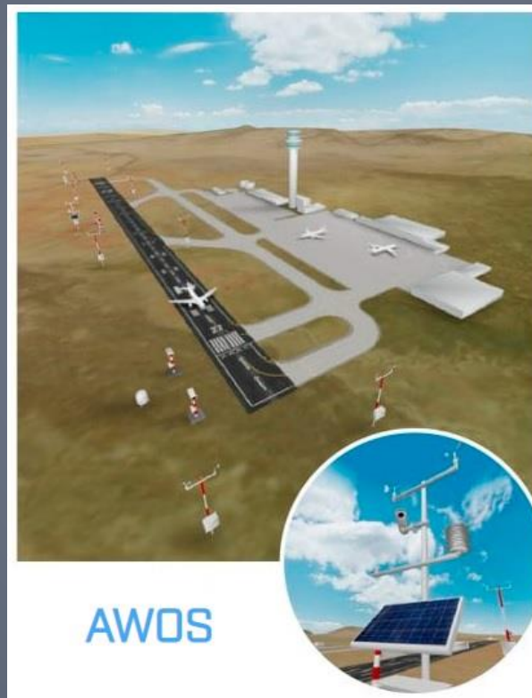
AWOS – Automated Weather Observation System
