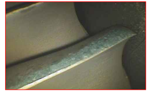
Compressor Turbine Blades Leading edge– Carbon erosion
