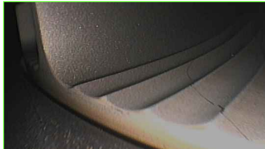
Impeller exducer – distal borescope probe mark
