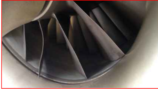
Engine noise Compressor 1 st stage rotor – Whistling
